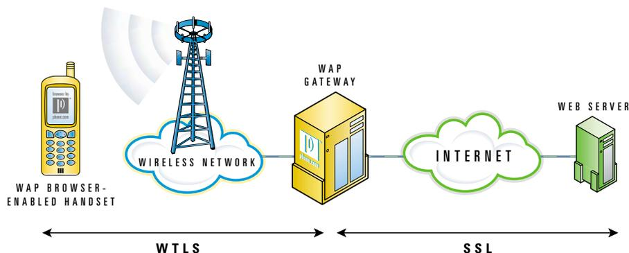
On the left side of Figure 2, the WAP gateway takes SSL-encrypted messages from the Web and translates them for transmission over wireless networks using WAP's WTLS security protocol. Messages from the handset to the Web server are likewise converted from WTLS to SSL. In essence, the WAP gateway is a bridge between the WTLS and SSL security protocols.
